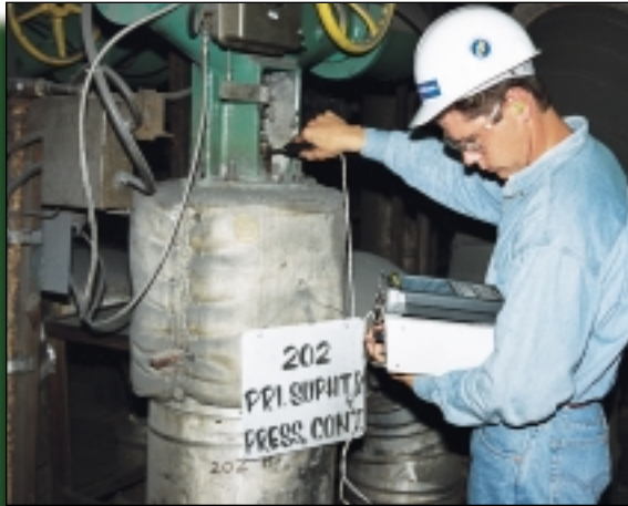
Figure 11: B&W's valve testing service can quickly detect even the slightest seat leakage with high accuracy.
