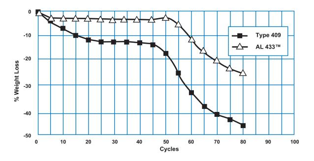
**Cyclic Oxidation/Corrosion Test**
