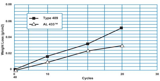
**Condensate Corrosion Test**
