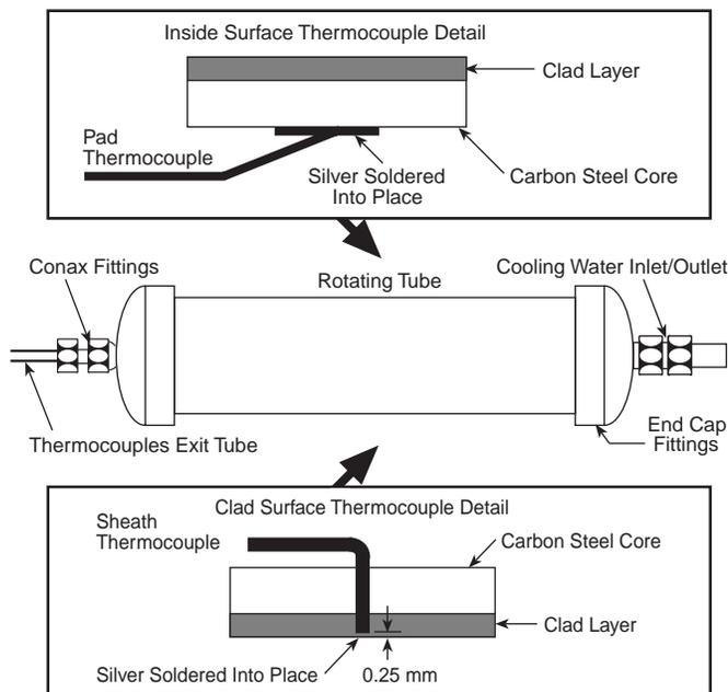
Figure 13 Test facility – thermocouple assembly.
