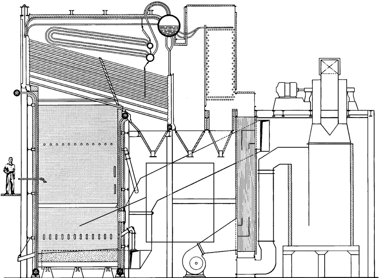
**Figure 1** World's first Tomlinson Recovery Boiler.
